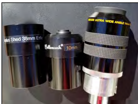
Figure 4. A basic knowledge of eyepieces is required for useful observing. Smaller focal length eyepieces offer greater magnification over higher focal length eyepieces. Eyepieces also vary in field of view, lens quality and eye relief. Shown here is an assortment of 2-inch barrel eyepieces.
