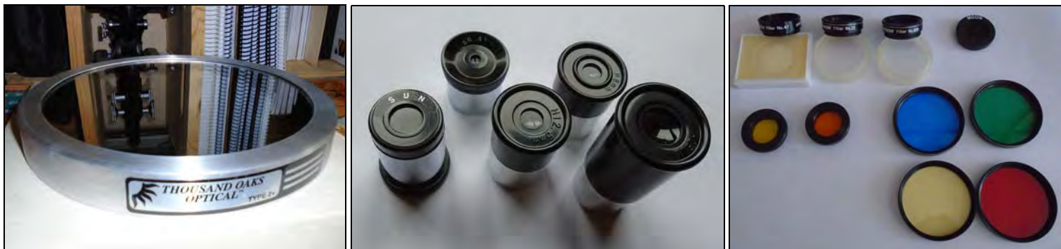
Figure 3. Solar, planetary and lunar filters exist for the enhancement of certain details. Above left , this Thousand Oaks solar filter fits over the front aperture of an 8-inch telescope. This one is used for visual observing, but others exist for photographic purposes. Above center , small eyepiece 0.965-inch solar filters are rarely seen anymore because of safety concerns. These filters, such as the one above at the left, screw into the threads on the back of eyepieces. Rather than the filter being fitted to the aperture end of the telescope, the filter receives the focused concentrated solar rays. Smaller type low-cost eyepieces are still readily found and can be used with adapters on all telescopes. Above right , this set of various size eyepiece filters can be used for lunar and planetary viewing.
