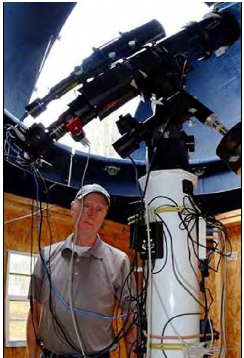
Figure 3. Jerry Hubbell at the Mark Slade Remote Observatory. Main instrument: 6.5-inch Explore Scientific 165 FPL-53 ED APO Carbon Fiber mounted on an Explore Scientific/Losmandy G11 PMC-Eight GEM. (Photo courtesy of Bill Paolini).
