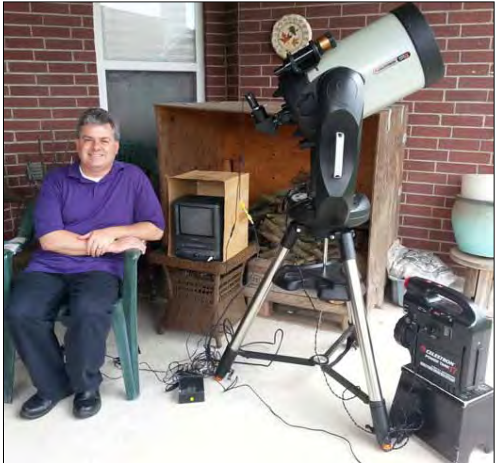
Brian Cudnik with his "family" of Lunar Meteoritic Impact Search equipment. His setup for doing lunar meteor observations and stellar occultations consists of a Celestron 11-inch telescope, a KPC-135 low light video camera (similar to Watec 902H), a KIWI-OSD with a GPS time inserter, and finally a TV-VCR combo
