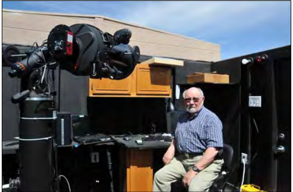
Figure 1. Wayne Bailey in March 2019 at his Tucson, AZ, observatory with his C-11 equipped with an SBIG STF-8300M CCD camera & filter wheel.
