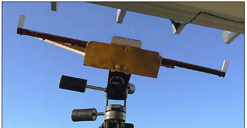
Figure 6. The dichotometer, mounted on a triaxial tripod to measure the elongation of a waning quarter-Moon.
