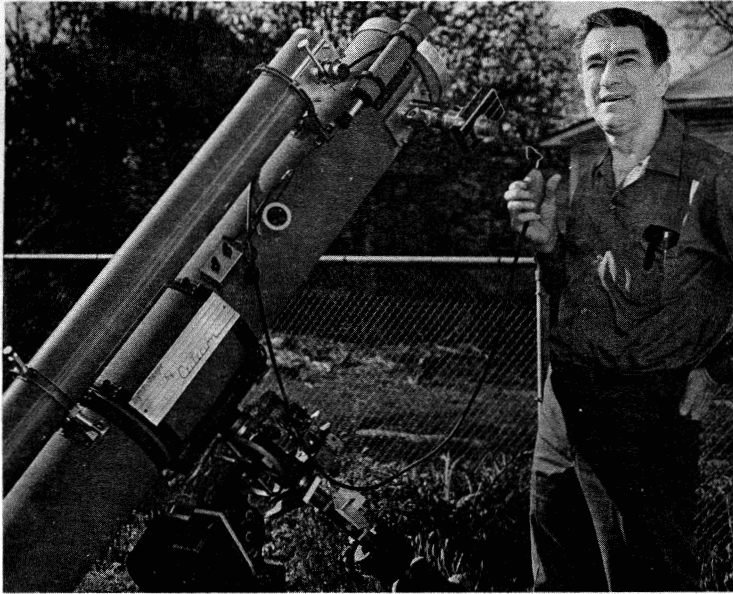
Figure 2. ALPO astrophotographer, Howard F. Zeh, of Temperance, Mich. with his reflecting 8-inch (20cm) f/8 Newtonian telescope with an 8 inch Byers RA Drive, a 4½-inch f/13 seeing monitor reflector, and an air-bulb shutter of vintage ca. 1888. Shown below, is an Argus C-3 35mm camera with various f-ratio eyepiece projection tubes and an 8mm Clavé Flossl ocular that Mr. Zeh uses to acquire quality planet photos which he so kindly contributes to ALPO Planet Section Recorders for their measurements and analyses.
