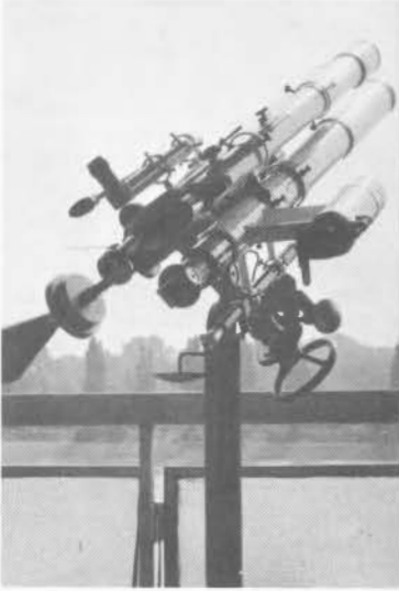
Figures 11 (left) and 12 (above). Four refractors on one mounting at the "Georgiana" Lunar Observing Station of the Research Group on Planetary and Geophysical Volcanology, Budapest, Hungary. Photographs supplied by Dr. Péter Hédervári. See text on page 110.
