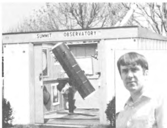
Robert A. Yajko & Observatory at Leechburg, Pa. has 250mm f/5 Newt. refl. and 106mm f/15 refr. that are used for systematic tricolor filter observations.
