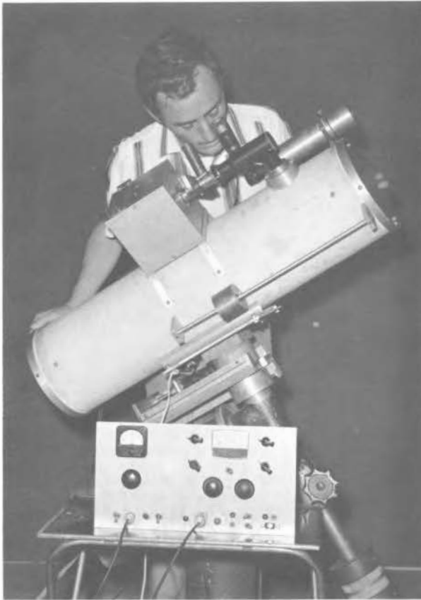
Figure 10. Photograph by Dennis Milon of R.B. Minton using his 6-inch, f/5 reflector in Tucson, Arizona. He employs a photoelectric photometer to determine the diameter and stellar magnitude of comets, such as 1969g. Instructions for building this photometer for $50 to $100 were given in JALPO, Vol. 24, Nos. 1-2, pp. 14-18.
