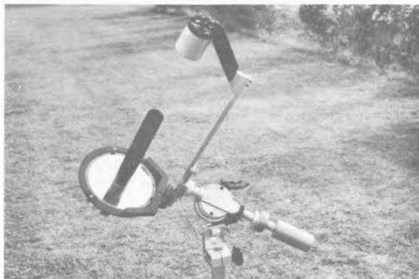
Figure 15. A light-weight 8-inch Cassegrainian designed and built by Victor Nikolashin. See his text on page 204.
