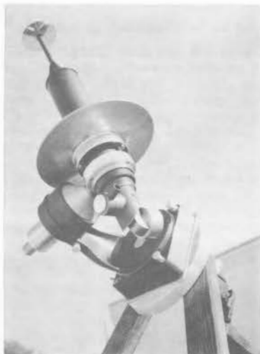
Figure 18. Light-weight 12-inch Cassegrain designed and built by Victor Nikolashin. The front secondary is here mounted in the center of the light-shield tube.
