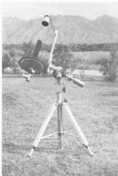
Figure 15. A light-weight 8-inch Cassegrainian designed and built by Victor Nikolashin. See his text on page 204.
