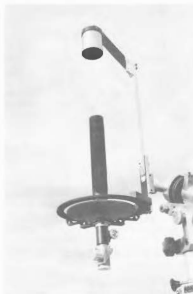
Figure 16. Closer view of optical components and their supports in Mr. Nikola-shin's 8-inch Cassegrainian reflector. One support rod holds entire telescope to equatorial mounting.
