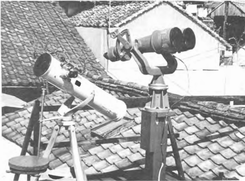
Figure 11. The altazimuth-mounted 20 X 120 binoculars are supported by a wood pier. A cord supplies electricity for the heated dewcaps, which prevent fogging of the objectives. To the left is a 15-centimeter f/6.3 reflector having a 2^{\circ}.5 field at 27X.
