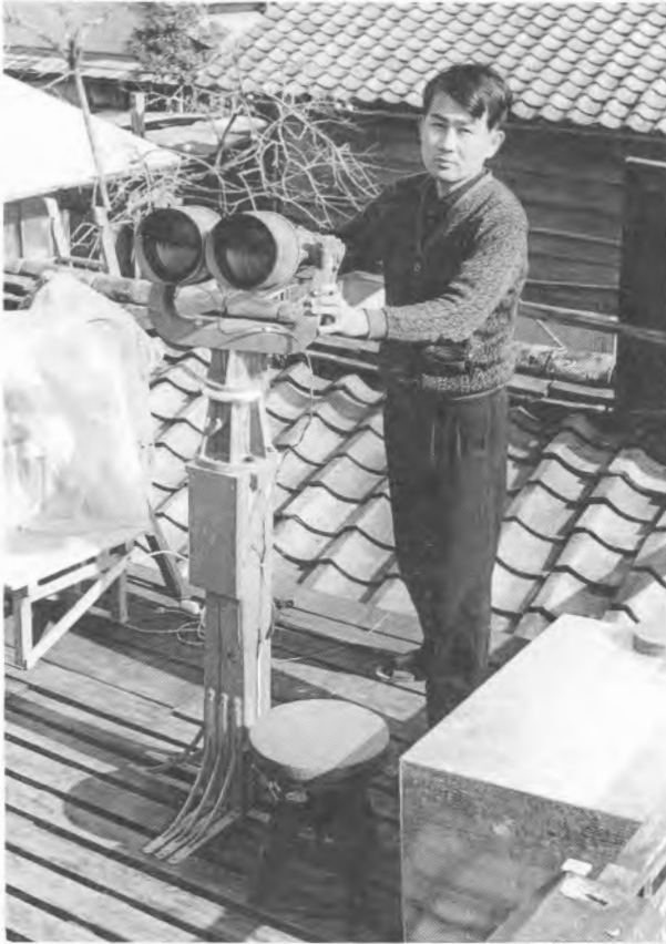
Figure 10. On a rooftop observing platform, Tsutomu Seki stands beside the 12-centimeter (5-inch) 20-power binoculars that were used in discovering Comet Seki 1967b on February 4, 1967. These binoculars have a field of three degrees.
