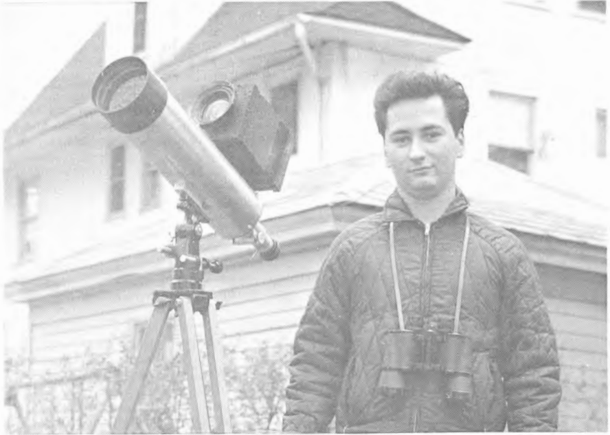
Figure 15. John Bortle, Mount Vernon, New York, who is one of the Comets Section's most active observers. He is shown with his comet observing equipment: 10X50 binoculars and 5-inch f/5 refractor with an Aero Ektar lens on the tube. Mr. Bortle also uses a 6-inch Rich-est Field Telescope. He writes comets reports for The Eyepiece of the Observing Group of the Amateur Astronomers Association, New York City.
