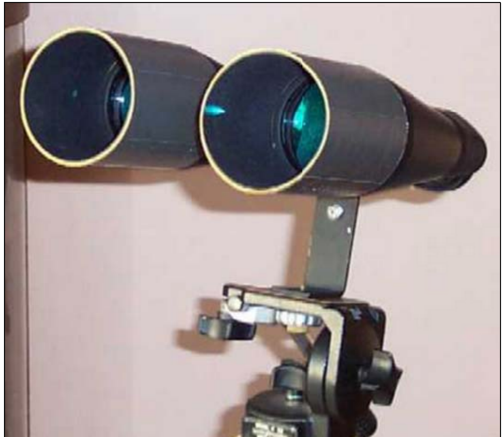
Figure 2. Giant binoculars with homemade dewshields attached. Image source: http://www.astromart.com/common/image_popup.asp?image=/images/forums/41000-41999/41461.jpg&caption=
