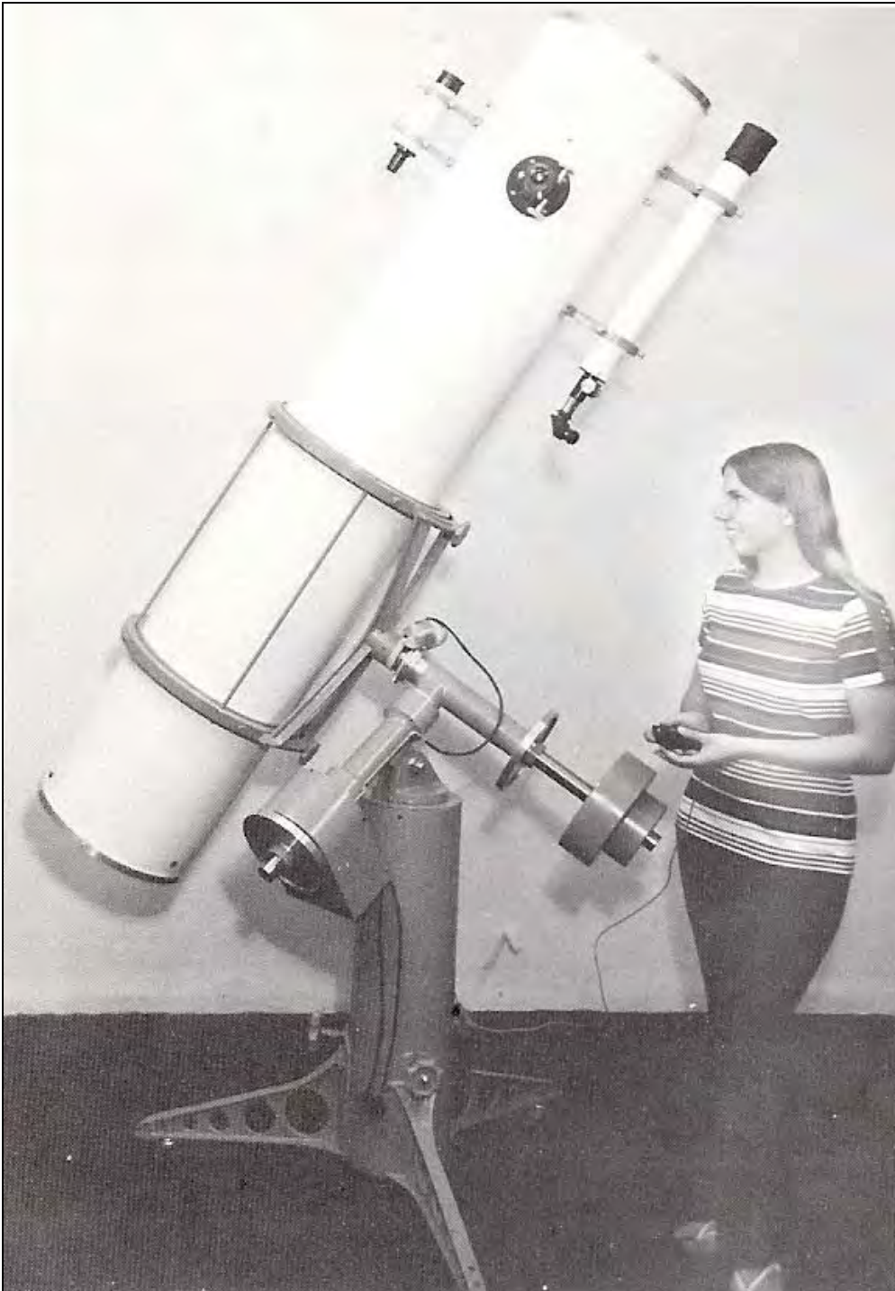
Figure 2: The Cave Optical Company’s 12.5-inch “transportable” Newtonian embodied the limitations of the traditional design.
