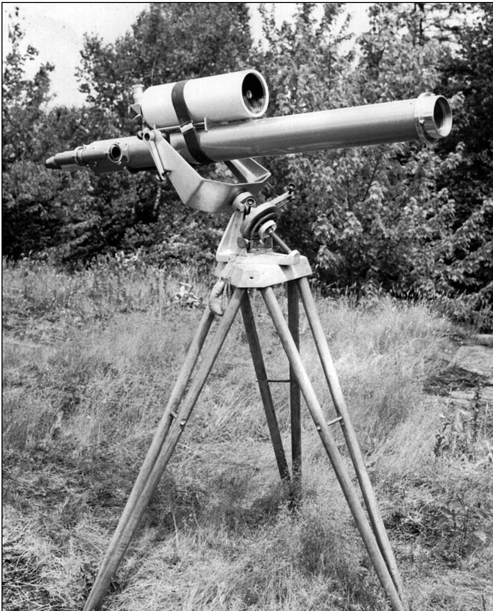
Figure 5: A 5-inch f/20 Maksutov made by John Gregory riding piggyback atop a 4-inch refractor. This compact instrument created a sensation when it was displayed at the 1956 Stellafane convention.
