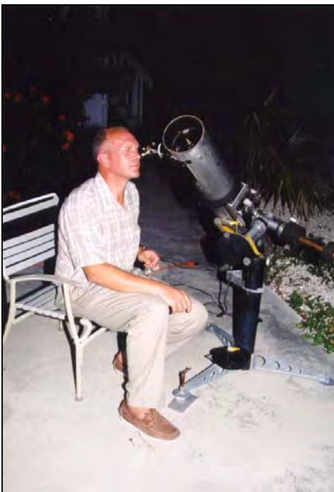
Figure 7. Tom Dobbins at the eyepiece of Don Parker’s venerable 6-inch f/8 Newtonian reflector, a classic instrument that provided excellent images of Mars.
