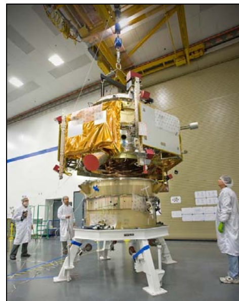
Figure 1. LCROSS Shepherding Spacecraft being lowered onto lower adapter ring, which connects it to the Centaur Upper Stage. (Photo credit: NASA, courtesy of Northrop Grumman)
