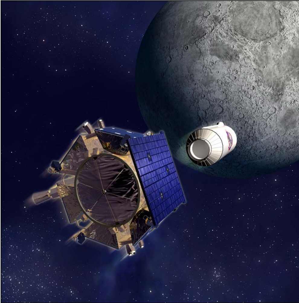
Figure 3. Impactor/Shepherdling Spacecraft Separation. The Shepherdling Spacecraft will trail the Impactor by several minutes to observe the impact and debris plume before it also impacts the Moon. (Note that the Moon's phase shown here is not the same as at the now-scheduled time of impact.) (Credit: NASA/Ames Research Center)
