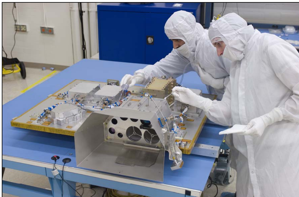
Figure 2. Shepherd Spacecraft instrument package. The instrument viewing apertures are visible within the sunshade. (Photo credit: NASA Ames Research Center/Dominic Hart)
