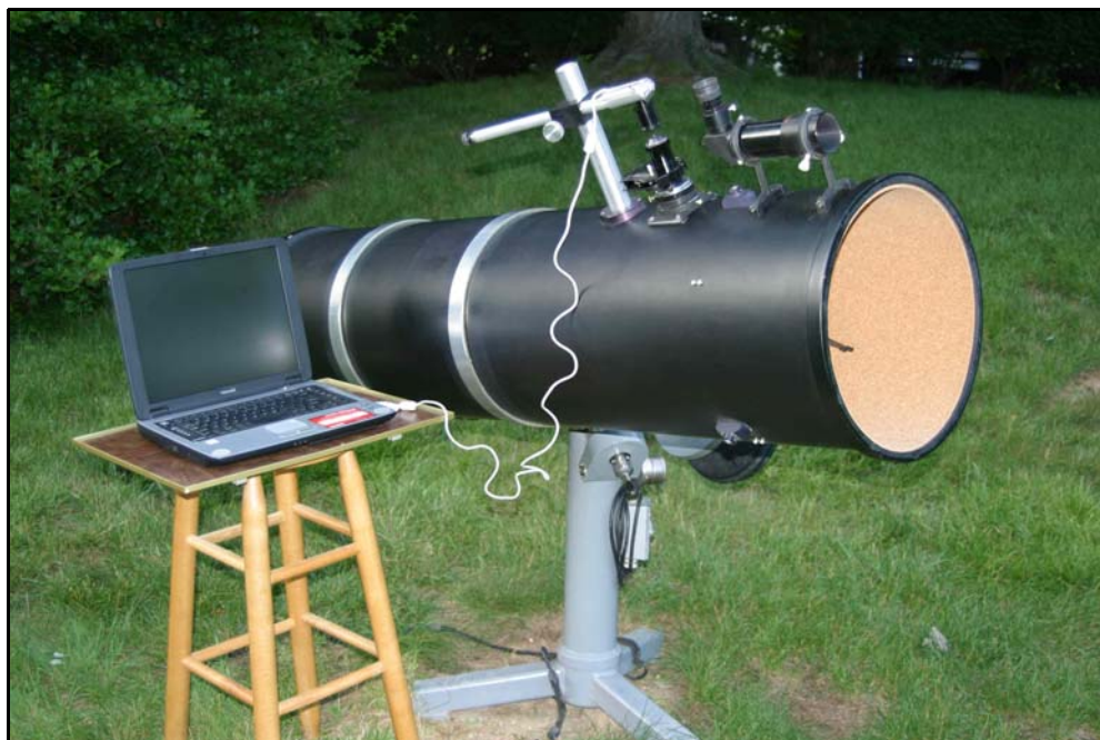
Figure 1. Imaging setup by Jim Melka, including laptop computer and 12.0 in. (30.5 cm) Newtonian reflector on German Equatorial Mount with a Philips ToUcam webcam configured for eyepiece projection; laptop equipped with K3CCD Tools image acquisition software, Registax 4.0 image processing software. (Image by Jim Melka)
