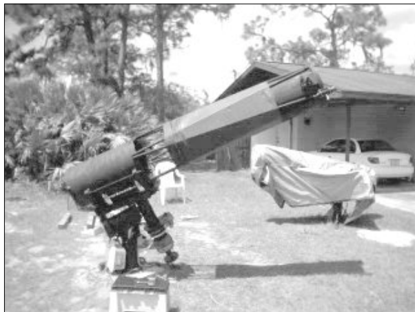
Beish equipment ready and steady: at left, 16-inch, f/6.9 uncovered and ready for use; at right, 12.5-inch, f/7 covered with IR blocking tarp.
