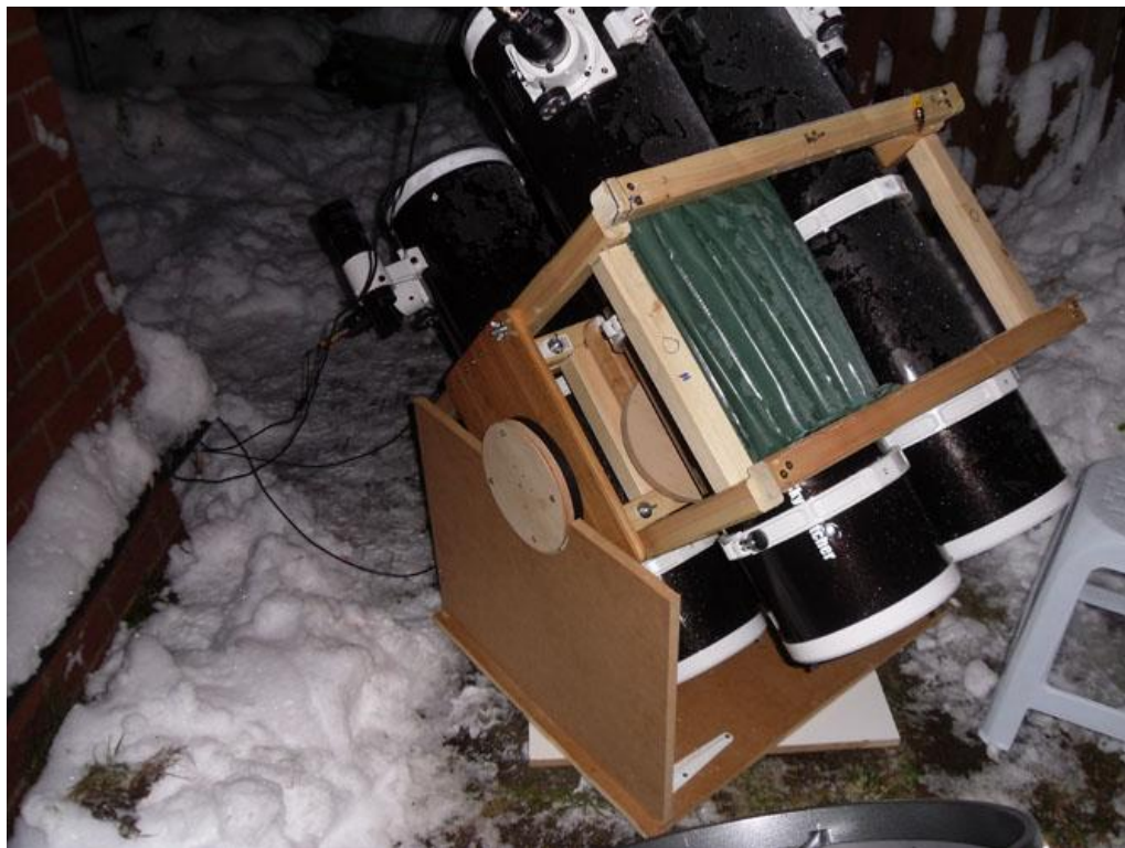
Figure 1. Four 8" f/5 Skywatcher tubes bolted together, on independent platforms with each scope operating in the following wavebands: ZWO CCD Filters: Red, Green, Kodak Wratten 87C near IR filter, and a low resolution diffraction grating. Purpose: Multi-waveband impact flash observing.
