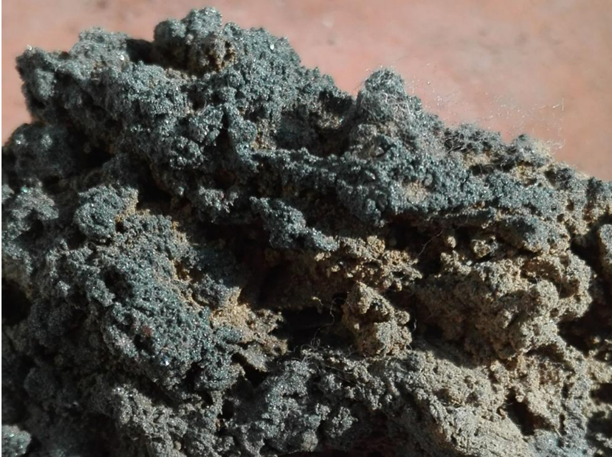
Figure 4: Siderazot (Fe 5 N 2 ) was found for the first time by Arcangelo Scacchi (1887) at Vesuvius, on the slag of the lava of 1884-85. The Siderazot which is presented in iridescent patinas with metallic reflections has also been found on the dross of other eruptions (1858, 1898, 1900, 1913, 1917, 1929 and 1944). It is probable that this mineral is formed by sublimation on high temperature slags (Lena private collection).
