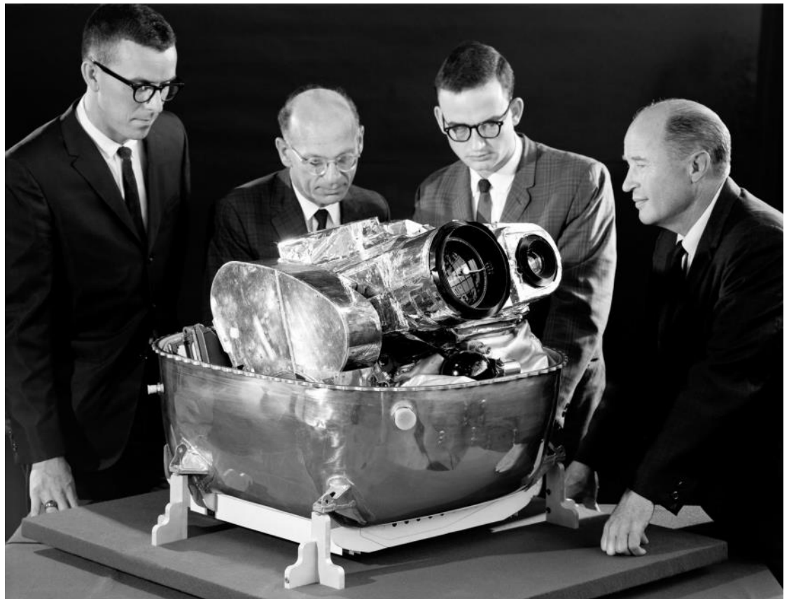
05 camera system.jpg The Lunar Orbiter camera system was originally developed by the Eastman Kodak company for the Air Force Samos reconnaissance satellite in the early 1960s. Photo by the Eastman Kodak company
