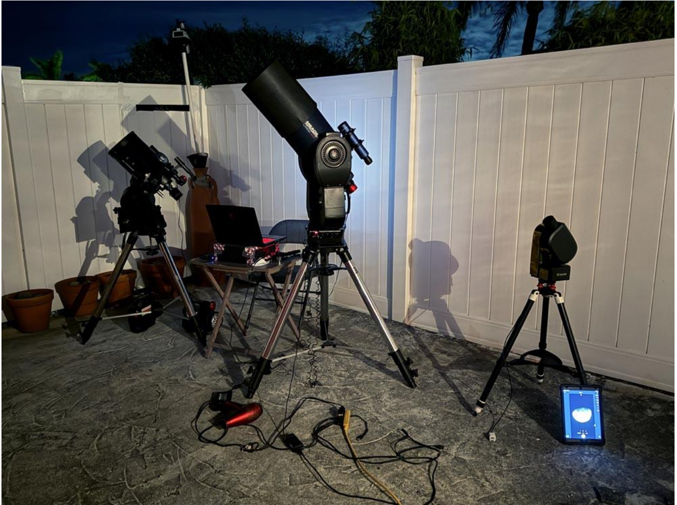
Figure 4: Equipment utilized. Right: Seestar S50 Smart Scope, center: Meade LX200GPS ACF 8-inch SCT, middle: MSI GF65 laptop computer Intel i7 with 6 cores 12 threads and 40GB of RAM, left: Meade 60mm refractor piggy-backed on a Meade LX6 8-inch SCT Ambient Weather WS8480 Falcon Weather Station.
