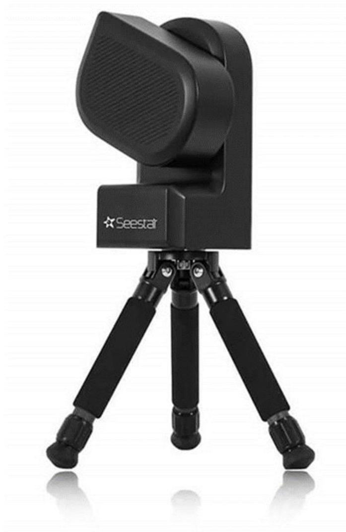
Figure 1: This smart scope features a 50mm triplet apochromatic lens at a focal length of 250mm at f/5. The sensor is a SONY IMX462MC color CMOS chip with a resolution of 1096 x 1936 pixels (2.1MP) at 2.90 microns. The SeeStar has added features such as a built-in dew heater as well as an internal UV-IR cut filter and dual band H-alpha and OIII light pollution filter. The telescope weighs only 3kg or 6.6 lbs. The SeeStar comes complete with a custom fit carrying case, carbon fiber tripod, solar filter, USB-A to USB-C charging cable and Quick-start guide all for only $499. Credit: ZWO website. See the ALPO Observers Notebook at https://soundcloud.com/observersnotebook where I recently recorded a podcast regarding the use of the SeeStar as a research instrument for ALPO.
