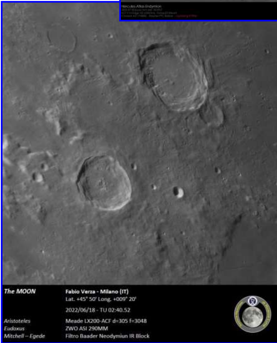
Aristoteles , Fabio Verza, SNdR, Milan, Italy. 2022 June 18 02:40 UT. Meade LX200 12 inch Schmidt-Cassegrain tele- scope, Baader Neodymium IR block filter, ZWO ASI290MM camera.
